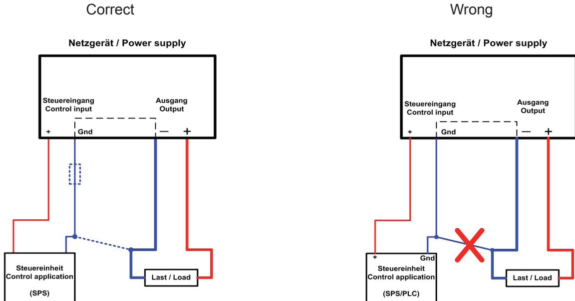
In order to measure the voltage at the load, use and wire the „Remote sense“ feature. The actual value output UMON, represents the voltage on the load and can be wired with the control application to measure the voltage. This prevents the current flowing via the control resp. measure lines.
