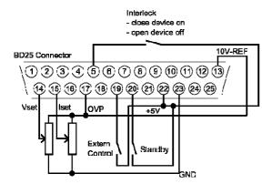
All digital outputs are OC outputs with a pull-up resistance after + 5 V. All analog inputs and outputs can be operated in 0-5 V or in 0-10 V mode.
