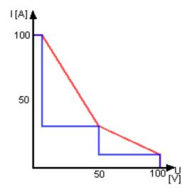
If output voltage or output current is changed afterwards, the characteristic keeps its course. Though values are stretched or compressed to the new range.
