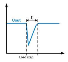
Example for pos. load step: the DC output will collapse below the adjusted value for a short time. t = transient time to settle the output voltage.
