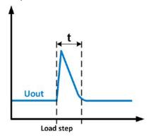
Example for neg. load step: the DC output will rise above the adjusted value for a short time. t = transient time to settle the output voltage.
