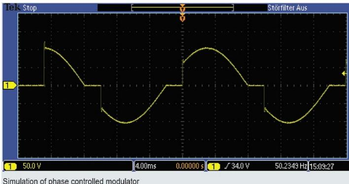
Simulation of phase controlled modulator
